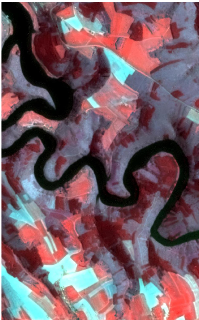
Processed image on Luxembourg after PAN sharpening, based on PRISMA satellite imagery – 5 meters resolution
